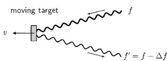
Fig. 8. Principle of Doppler velocimetry: a laser beam reflected by a moving object returns with a frequency change,  $\Delta f$ , known as Doppler shift. The velocity,  $v$ , can be determined from  $\Delta f$ . (Reproduced from Bebie, 1995 with permission.)
